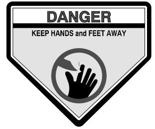
For Units with a Blade Brake Clutch PART NO.: 43-8480 LOCATION: Top RH Surface of Mower Deck
